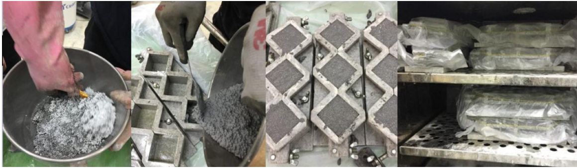
Figure 1. Mixing and curing process
