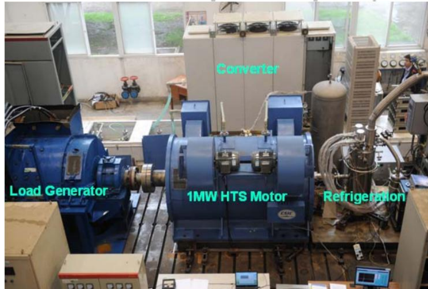
Figure 7: 1MW HTS motor test bed
