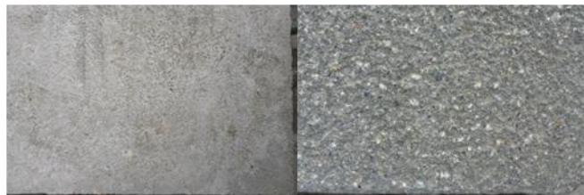
(b) Smooth(left) and roughened(right) surfaces
