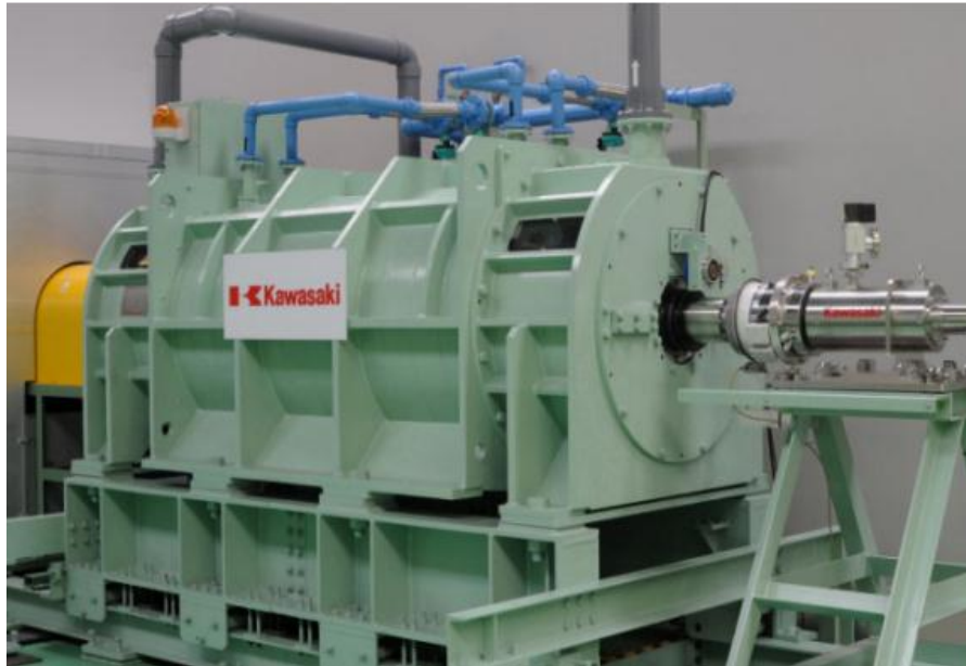
Figure 6: 1 MW class superconducting motor for ship propulsion of Kawasaki
