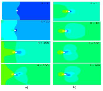
Figure 4: Static pressure distribution of water flow a) Case 1, b) Case 2
