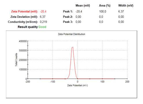
Figure 5: Zeta potential determination by dynamic light scattering (DLS)
