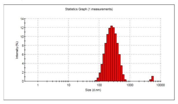
Figure 4: DLS analysis results of in vivo synthesized Ag NPs
