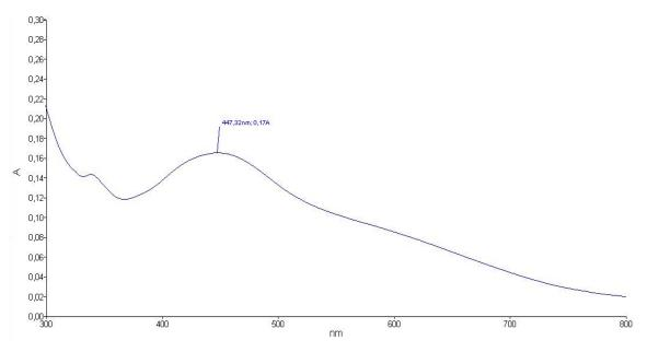
Figure 2: UV-Vis absorption spectra of in vivo synthetized AgNPs.
