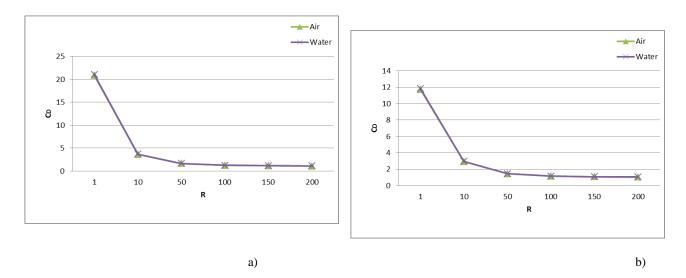
Figure 7: Drag coefficient versus with Reynold number a) Case 1, b) Case 2
