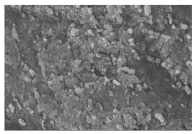
Figure 6: SEM image of in vivo synthetized AgNPs
