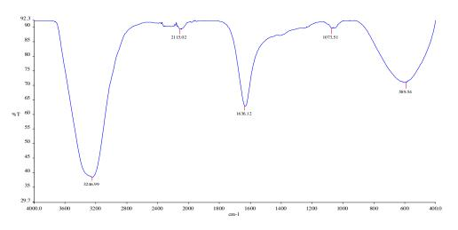
Figure 3: FT-IR spectrum of in vivo synthetized AgNPs.
