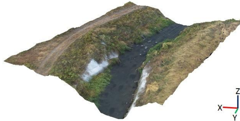
Figure 10: 3D textured map built from the solid model showing the geometry and the texture of the environment around the river
