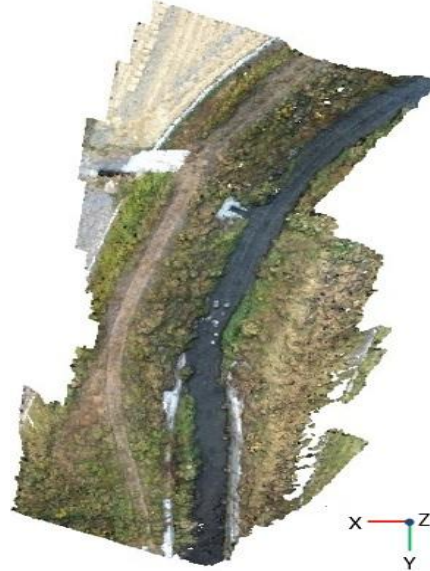
Figure 8: Dense point cloud built from the estimated positions and orientations of the twenty-seven photo images and the sparse point cloud
